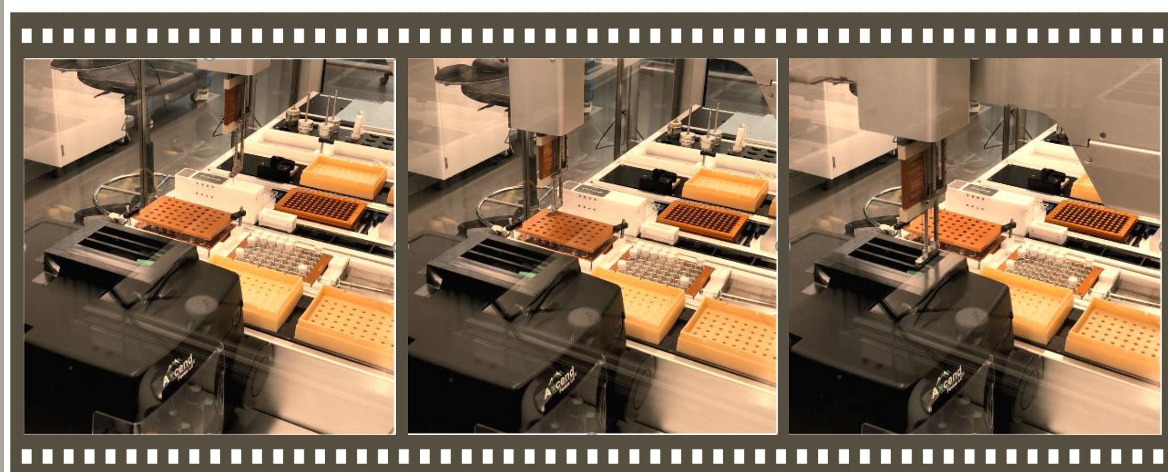
Figure 2. The extendable syringe needle on the CM3 robotic platform draws liquid from a plate and injects the sample onto the Axcend FocusLC.
