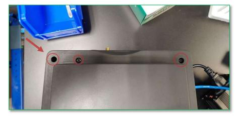
6. Ensuring all seven screws have been removed, press and hold down the green button on the handle and simultaneously lift top paneling to carefully remove the Focus LC top cover.
