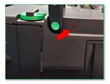
5. Remove the three screws located on top of the Focus, towards the rear of the instrument. While the center- and right-most screws (9mm, rounded head) are easily
