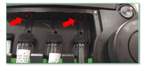
4. Remove the two horizontal screws (10.5mm, flush head) on each side of the instrument, underneath the handle.
